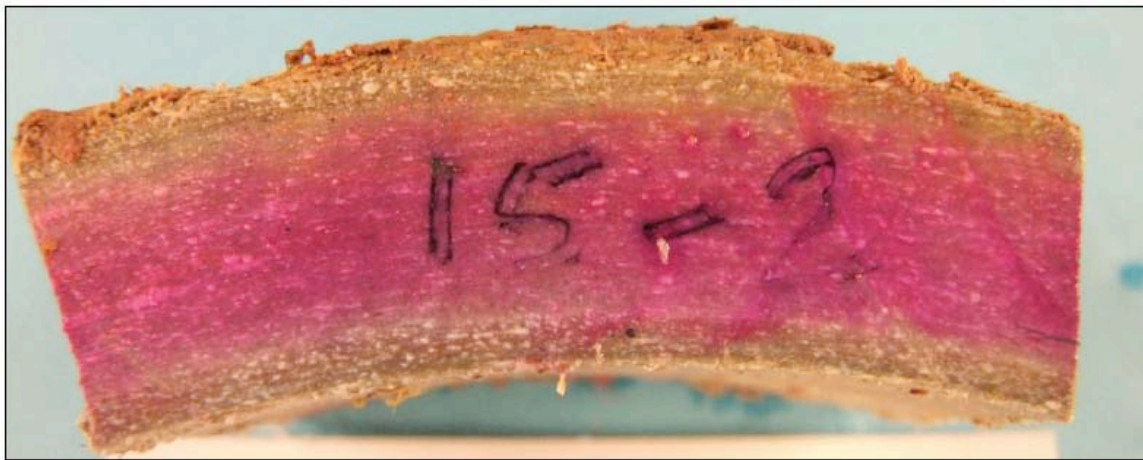
Figure C-1. Results of Stain Test, EBMUD AC pipe
